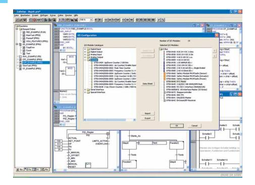
WAGO-I/O-PRO is a programming and visualization tool for control programs. This software is used to develop PLC applications for WAGO-I/O-SYSTEM 750 Programmable Fieldbus Controllers.
